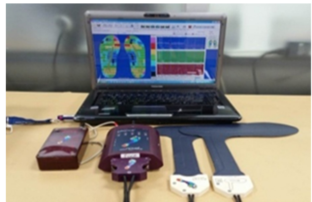
Fig. 1. Plantar pressure system (Pedar-X-32, Novel GmbH, München, Germany).
