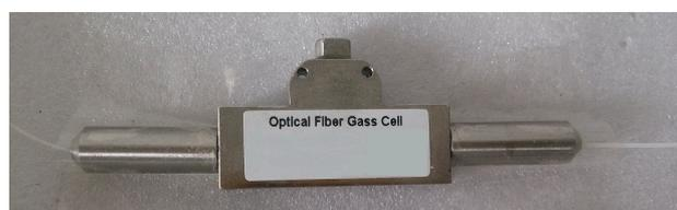
**Figure 4.** The gas cell structure.
