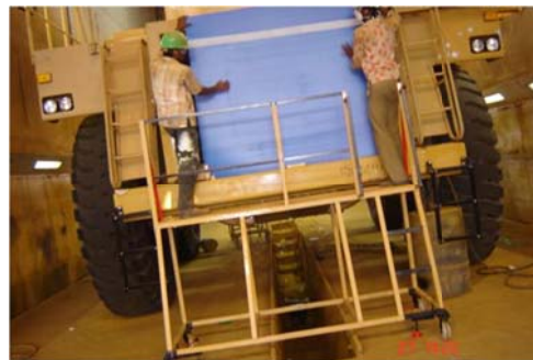
Figure 9. Masking with safety trolley-operator risk eliminated
