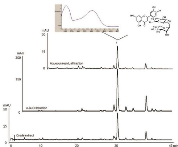
**Figure 1.** HPLC chromatograms of crude extract, aqueous residual fraction and *n*-butanol fraction of leaves of *M. x paradisiaca* with photo-diode array (PDA) detection at 340 nm. 1. rutin (rt 30.6 min).
