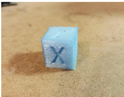
Figure 14. Calibration cube made of BPET.
