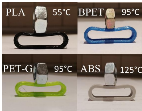
Figure 18. Samples at the initial stage of melting.
