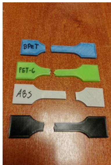
Figure 23. Samples after tensile test.
