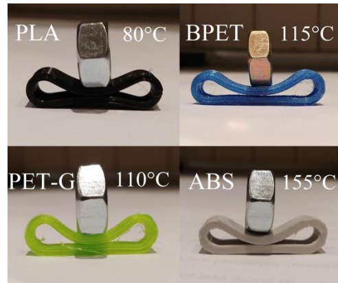
Figure 19. Completely melted samples.
