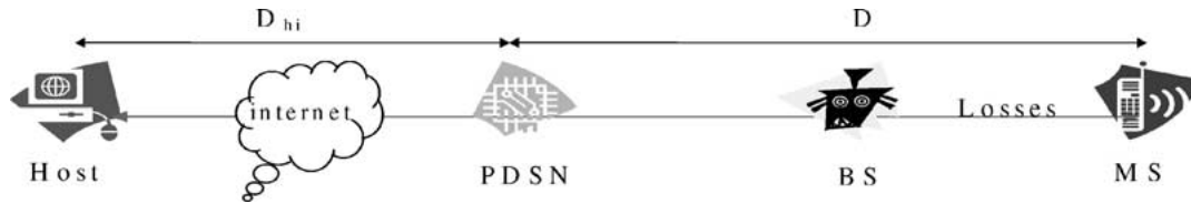
Figure 5. Modeling the communication network between the mobile and the host.
