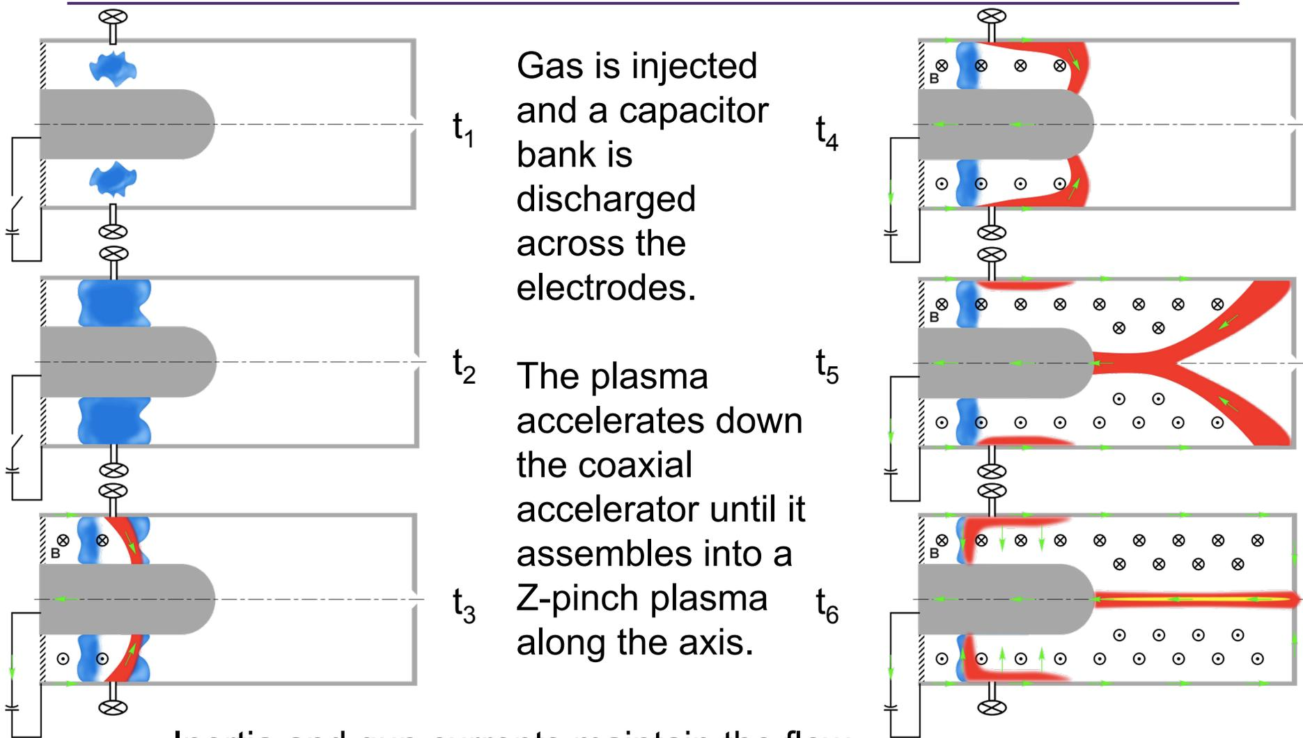
Inertia and gun currents maintain the flow until the accelerator plasma empties.
