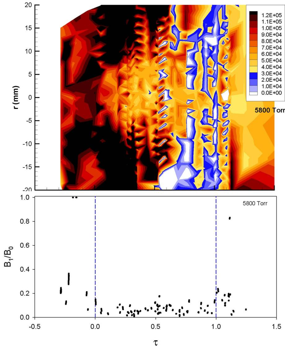
$\tau < 0$ , plasma assembly, the axial plasma velocity is high and uniform,  $v_z' \approx 0-4 \times 10^6 \text{ s}^{-1}$ .
