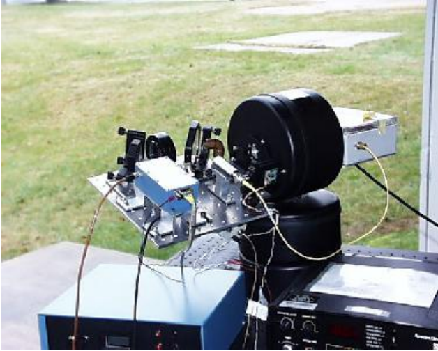
Figure 11. The transmit/receive assembly used in the NRL MQW field tests is shown. (a) The laser diode light is coupled into a fiber which is connected to the lens system. (b) The transmitted then retroreflected light is returned using a beam splitter and the signal is captured by a standard avalanche photodiode.
