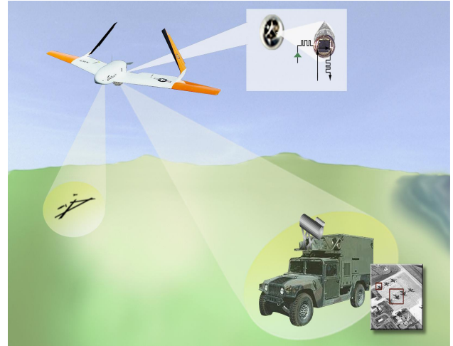
Figure 8. The MQW modulating retroreflector incorporated into an airborne reconnaissance concept using an Unmanned Aerial Vehicle is shown above. When configured into an array, the MQW modulating retroreflector concept significantly reduces the parasitic payload requirements for the onboard communications system.
