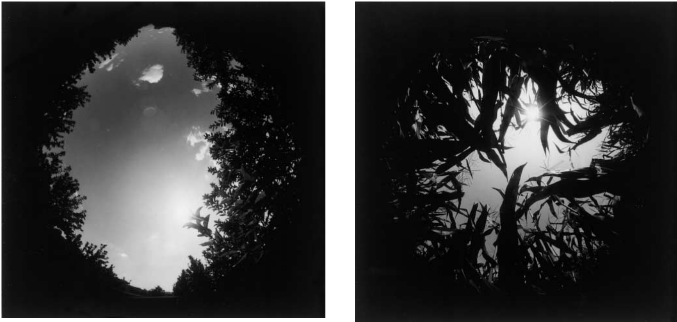
Fig. 1. Hemispherical photograph of a measurement site in the (left) orchard and (right) maize canopy. The centers of the photographs represent the zenith. Distance from the center toward the edge is linearly related to the zenith angle.
