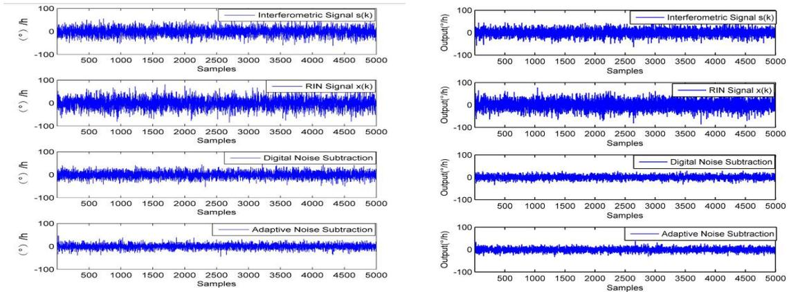
(a) Effects of two noise subtraction methods at 10°C
