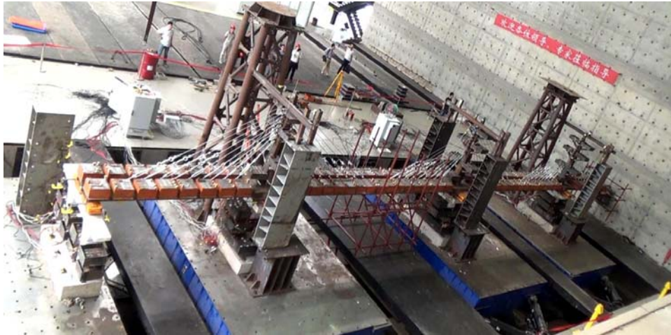
Figure. 6. Shaking table experiment model of Chao-yang bridge
