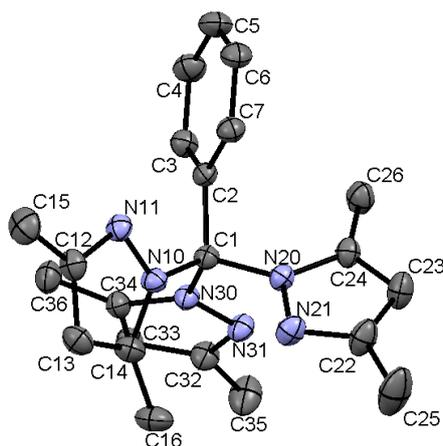
**Figure 2.** ORTEP perspective of compound **1a** at 30% probability level, hydrogen atoms are omitted for clarity. Selected bonds lengths (Å) and angles (°): N10-C1 1.4657(19), N20-C1 1.4725(18), N30-C1 1.479(2), C1-C2 1.532(2), N30-C1-C2 111.47(11), N20-C1-C2 107.84(11), N30-C1-C2 111.75(11), N10-C1-N20 109.86(11), N10-C1-N30 106.48(12), N20-C1-N30 109.43(11), N11-N10-C1 119.04(11), N21-N20-C1 118.72(11), N31-N30-C1 119.76(11).
