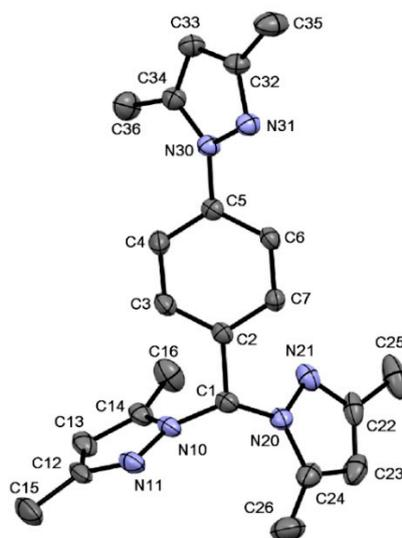
**Figure 4.** ORTEP perspective of compound 2 at 25% probability level, hydrogen atoms and the molecule of water are omitted for clarity. Selected bonds lengths (Å) and angles (°): N10-C1 1.464(5), N20-C1 1.445(5), C1-C2 1.521(5), N10-C1-C2 112.5(3), N20-C1-C2 114.1(3), N10-C1-N20 111.5(3), N11-N10-C1 116.7(3), N21-N20-C1 121.4(3).
