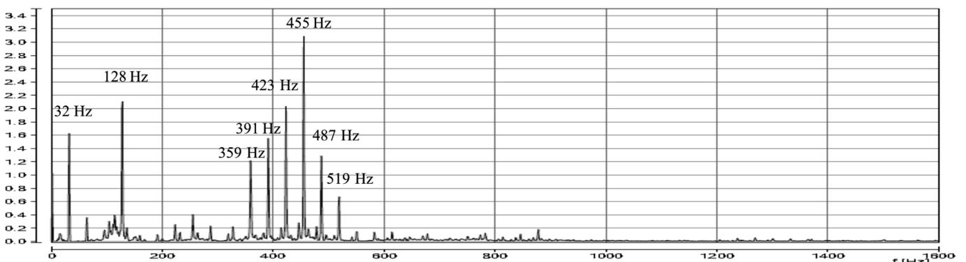
Fig. 12 : Vibration spectra (RMS value 5.4 mm/s)
