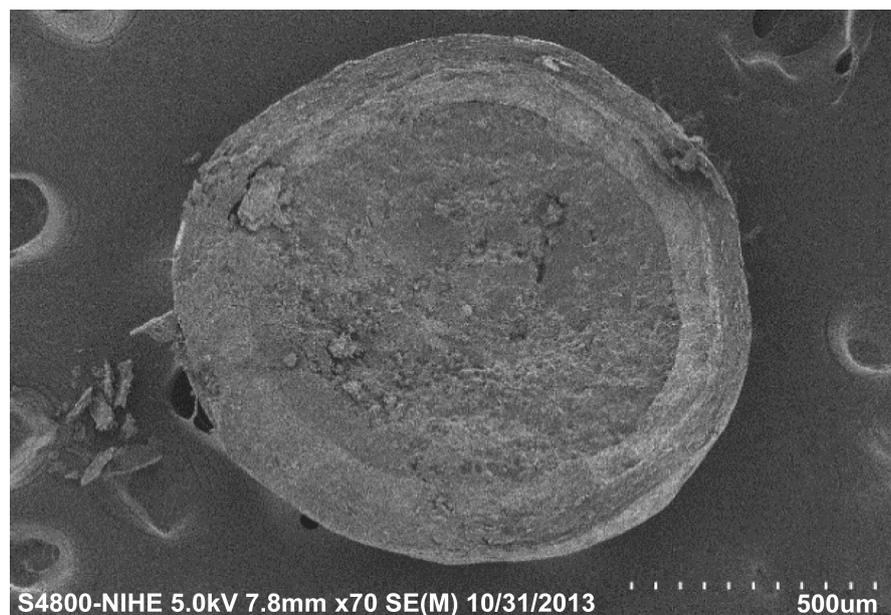
**Figure 4.** SEM of optimal formulation of LPZ enteric-coated pellets showing three coating layers around the sugar bead core.
