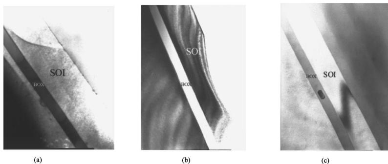
FIG. 1. Dependence of microstructure evolution on the energy for samples implanted with the oxygen dose of  $4.5 \times 10^{17} \text{ cm}^{-2}$  at the energies of (a) 160 keV, (b) 130 keV, and (c) 100 keV.
