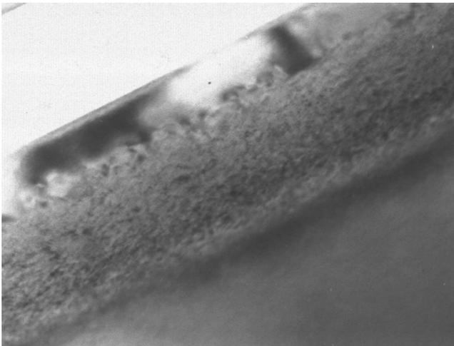
FIG. 4. Typical XTEM microphotograph of the as-implanted low-dose wafer likely to form a high-integrity BOX layer.
