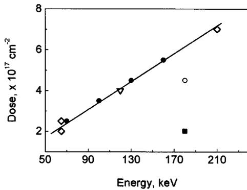
FIG. 3. Plot of a series of good dose-energy matches for the formation of high-quality low-dose SIMOX materials.
