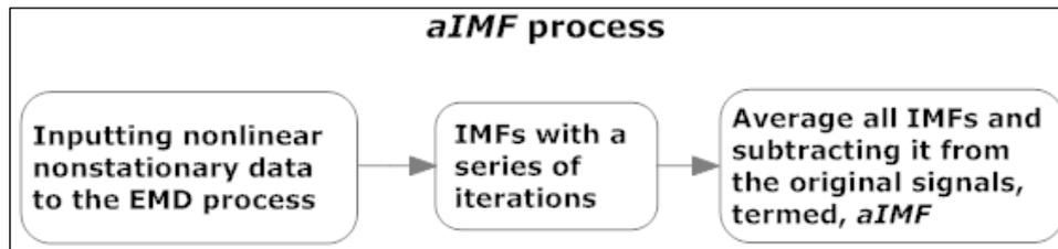
Referring to Figure 2, the proposed algorithm aIMF has an advantage which provides stoppage criteria once the two conditions of the EMD process defined in Section 2.1 are accomplished. This is because with more iteration, the more residual  $r_n(t)$  becomes either over-distorted or a monochromatic function from which no further IMF can be decomposed.
