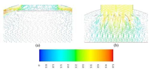
Figure 7. Velocity Vectors for (a) Unmodified and (b) Modified Designs
