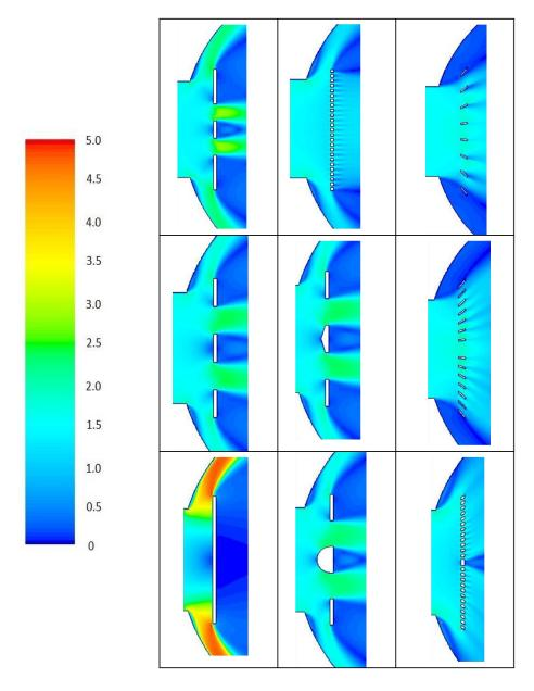
Figure 8. Velocity contours for modified plate designs
