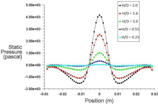
Figure 3. Effect of H/D ratio on the pressure distribution
