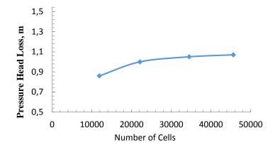
Figure 2(a). Grid independence test
