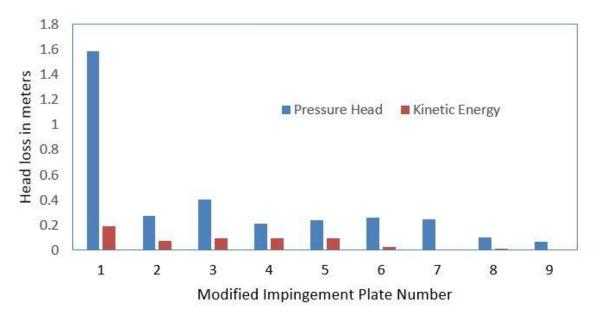
Figure 9. Kinetic and pressure head loss across different impingement plate geometries
