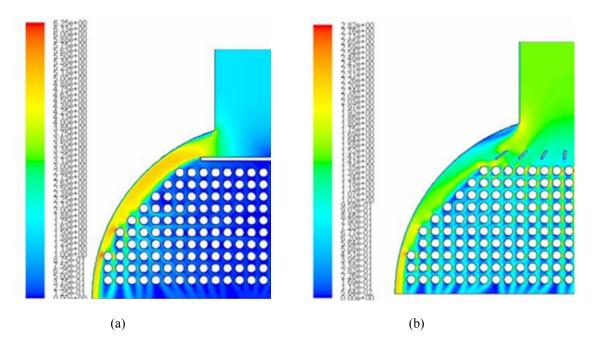
Figure 11. Velocity contours with (a) Unmodified (b) Modified Plate geometries
