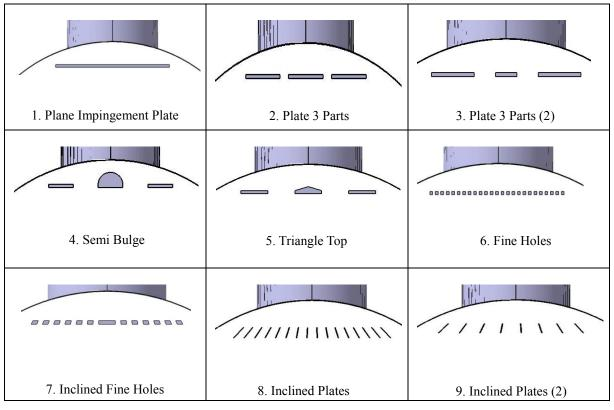
Figure 6. 2D Impingement plate geometries
