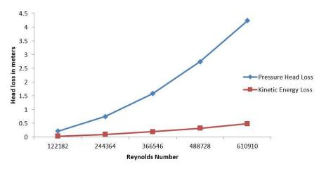
Figure 5. Variation of pressure head loss and kinetic energy head loss with Reynolds number
