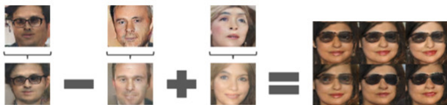
Figure 41. Example of smile arithmetic and arithmetic for wearing glass using GAN: a man with glasses minus man without glasses plus woman without glasses equal to woman with glasses.
