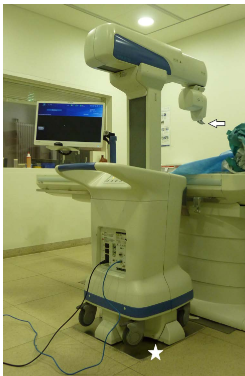
Figure 1. The experimental setup. The robotic device is mounted onto a docking plate (*) next to the CT table for spatial orientation. With the integrated planning computer access paths can be visualized by using a graphical user interface that supports multiplanar view angles. The white arrow marks the needle holding arm, which is then aligned to the planned trajectory. At the tip instruments from 11 to 24 gauge can be inserted through dedicated clamped adapters. The data cable, which is linked to the CT workstation and the power cord can be seen at the bottom of the image.
