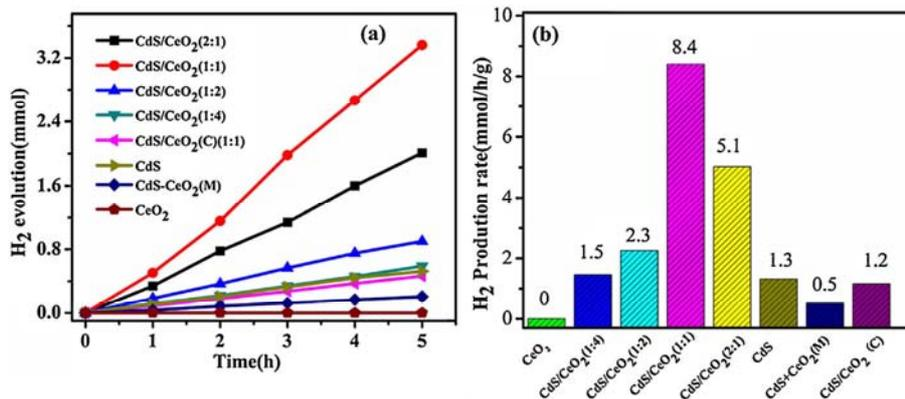
**Figure 5.** (a) Time-dependent  $\text{H}_2$  production performance, (b) rate of  $\text{H}_2$  evolution of bare CdS,  $\text{CeO}_2$  and CdS/ $\text{CeO}_2$  (n: m) nanocomposites under visible light irradiation.
