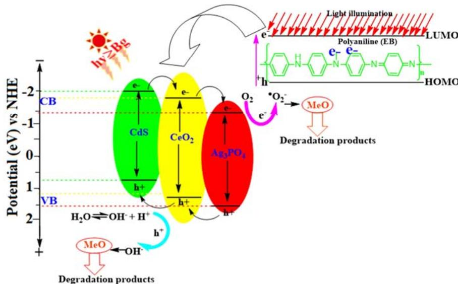
Figure 11. Mechanism of photocatalytic degradation of organic contaminant (MeO) by PAST photocatalyst under visible light irradiation.
