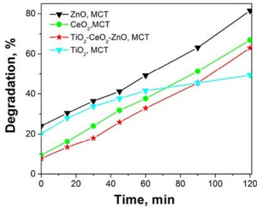
**Figure 9.** The degradation of the MO dye in water solution with the course of time under UV-A illumination at 464 nm using  $\text{TiO}_2$ ,  $\text{CeO}_2$ ,  $\text{ZnO}$  and  $\text{TiO}_2/\text{CeO}_2/\text{ZnO}$  photocatalysts.
