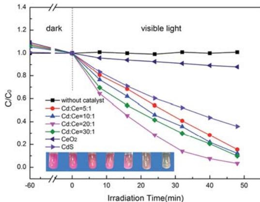
**Figure 4.** Effect of  $\text{CeO}_2$  loading on photocatalytic degradation of RhB; the suspensions containing 0.4 g/L catalysts, natural pH=4.3, initial concentration=40 mg/L,  $\lambda \geq 420$  nm.
