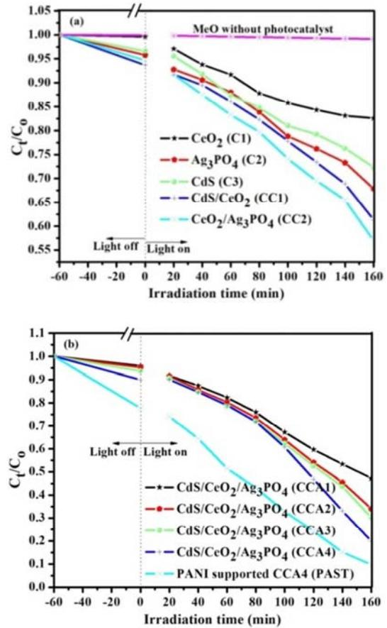
**Figure 10.** (a) Degradation efficiency of the as-synthesized photocatalyst [ $\text{CeO}_2$ ,  $\text{Ag}_3\text{PO}_4$ ,  $\text{CdS}$ ,  $\text{CdS}/\text{CeO}_2$  and  $\text{CeO}_2/\text{Ag}_3\text{PO}_4$ ] as function of visible irradiation time; (b) Photocatalytic degradation of the as-synthesized bare ternary and supported nanocomposite.
