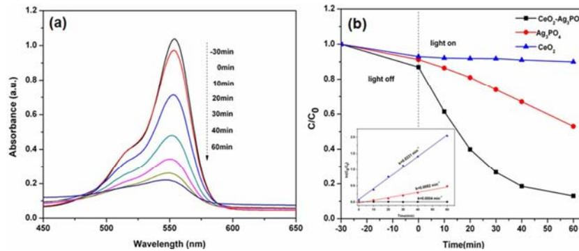
**Figure 2.** UV-Vis absorbance spectra of RhB solution after photocatalytic degradation with  $\text{CeO}_2/\text{Ag}_3\text{PO}_4$  heterojunction (a) and RhB concentration  $C_t/C_0$  and  $\ln(C_0/C_t)$  (inset) vs. time with  $\text{CeO}_2$ ,  $\text{Ag}_3\text{PO}_4$  and  $\text{CeO}_2/\text{Ag}_3\text{PO}_4$  (b) under visible light irradiation.
