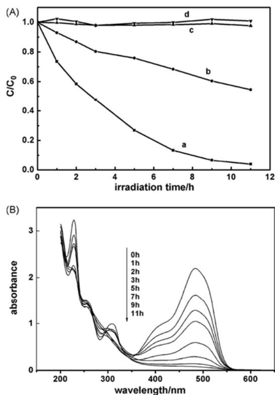
**Figure 1.** (A) Temporal course of the photodegradation of AO7 in CeO<sub>2</sub> aqueous dispersions under visible light irradiation: (a) CeO<sub>2</sub> under visible irradiation ( $\lambda > 420$  nm). (b) TiO<sub>2</sub> under irradiation ( $\lambda > 420$  nm). (c) No catalyst. (d) CeO<sub>2</sub> in the dark. (B) UV/Vis spectral changes recorded for (a) as a function of irradiation time.
