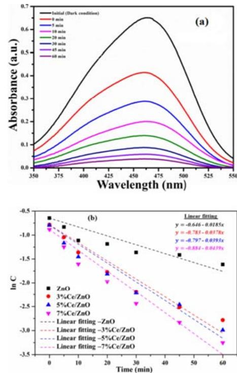
**Figure 8.** (a) Change in absorption spectra of the  $CeO_2/ZnO$  catalysts (b) First-order kinetic adsorption curves during photodegradation of methyl orange.
