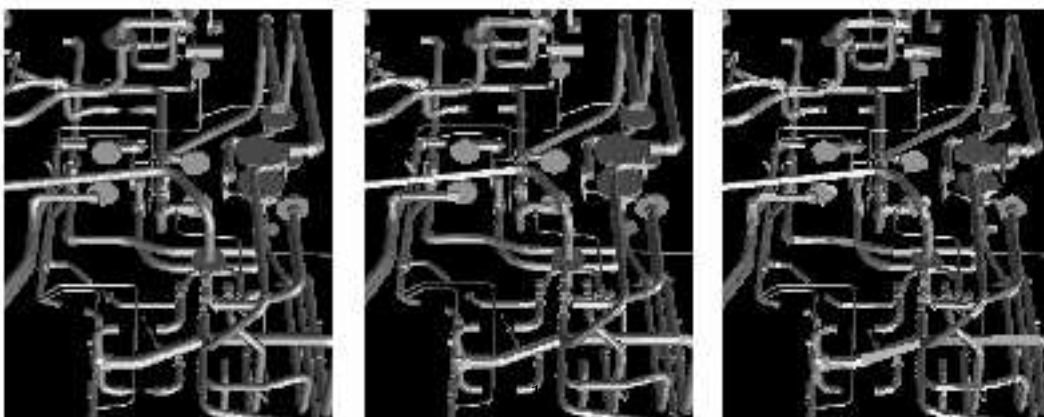
Figure 9: Side-by-side comparison of 3 levels-of-detail of a 625 object segment of the auxiliary machine room dataset. From left to right: 86,232 triangles, 31,486 triangles, and 12,788 triangles.
