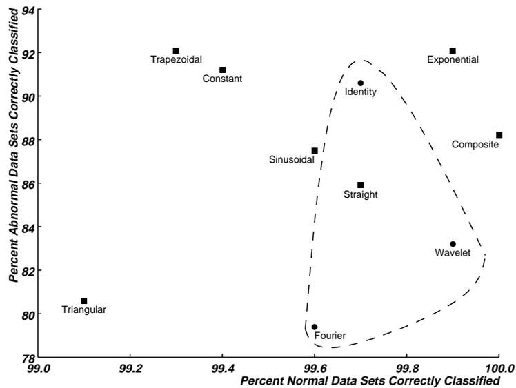
**Figure 4.14** The relative classification accuracies for all feature extraction methods for the 405 nm parameter. Each feature extraction method is plotted using the mean percent of normal and abnormal data sets correctly classified as coordinates. For the statistical feature extraction methods, the results with padding are used and are enclosed with a dashed line.
