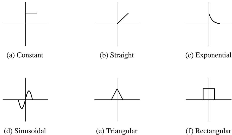
**Figure 2.6** Types of modulation commonly used by signal processing systems to transmit information via a continuous medium (e.g., an electrical current) include (a) constant, (b) straight, (c) exponential, (d) sinusoidal, (e) triangular, and (f) rectangular.
