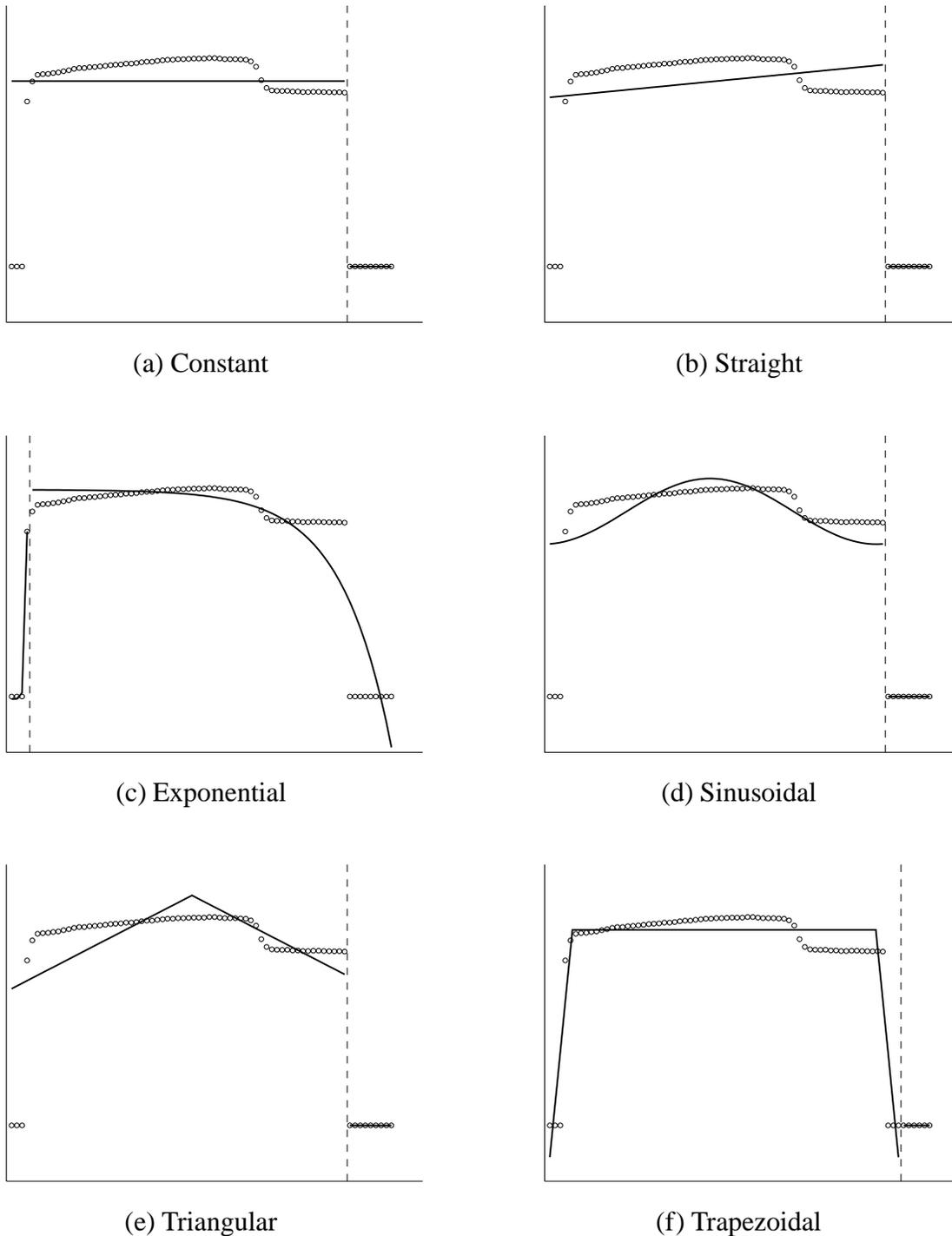
**Figure 3.2** The piecewise extraction of the six structures to fit two subregions to a common data set. Each graph shows the input time-series data plotted with hollow bullets overlaid with two solid lines, one for the structure extracted from each subregion, and a vertical dashed line separating the two subregions. The super-structures ordered from smallest to largest sum of squared error are (f) trapezoidal, (c) exponential, (e) triangular, (d) sinusoidal, (b) straight, and (a) constant.
