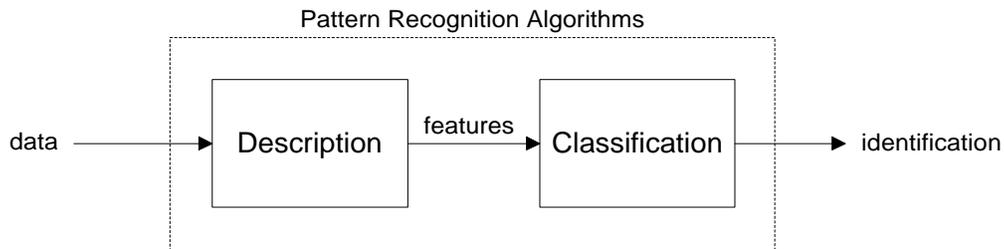
**Figure 2.2** The two separate tasks commonly used to divide the algorithms within automated pattern recognition systems. The description task transforms data collected from the environment into features. The classification task arrives at an identification based on the features provided by the description task.
