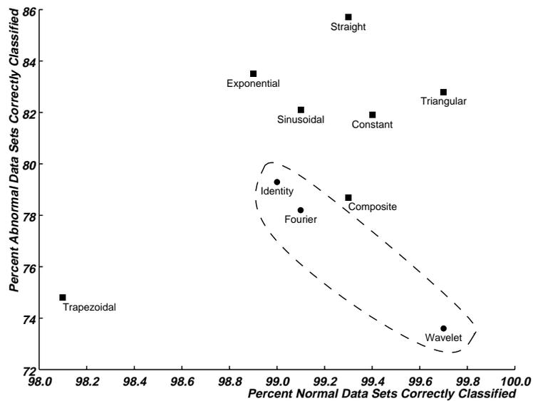
**Figure 4.15** The relative classification accuracies for all feature extraction methods for the 520 nm parameter. Each feature extraction method is plotted using the mean percent of normal and abnormal data sets correctly classified as coordinates. For the statistical feature extraction methods, the results with padding are used and are enclosed with a dashed line.
