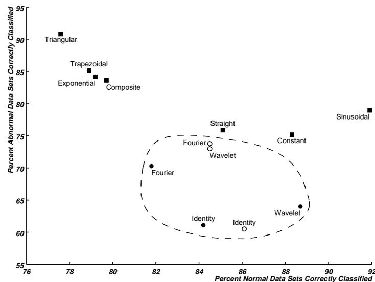
**Figure 4.17** The relative classification accuracies for all feature extraction methods for the lead 1 parameter. Each feature extraction method is plotted using the mean percent of the normal and abnormal data sets correctly classified as coordinates. A dashed line encloses the three statistical feature extractors for both types of data preprocessing: padding (plotted with solid bullets) and truncation (plotted with hollow bullets).
