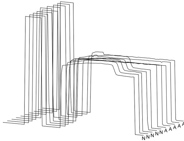
**Figure 4.8** Examples of normal and abnormal data sets for the 405 nm parameter in the wafer database. The waveforms labeled with “N” are graphical representations of five normal data sets, and the waveforms labeled with “A” are graphical representations of five abnormal data sets. These data sets were recorded simultaneously with those shown in Figure 4.9.
