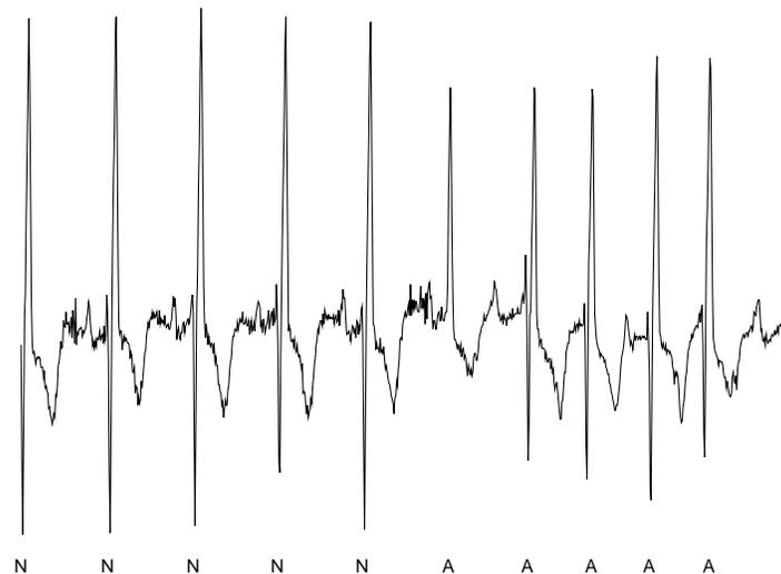
**Figure 4.11** Examples of normal and abnormal data sets for the lead 1 parameter in the ECG database. The graphical representation of five normal and five abnormal data sets are shown concatenated into one continuous waveform. A label appears at the onset of each data set within the waveform: an “N” indicates the start of a normal data set, and an “A” indicates the start of an abnormal data set. These data sets were recorded simultaneously with those shown in Figure 4.10.
