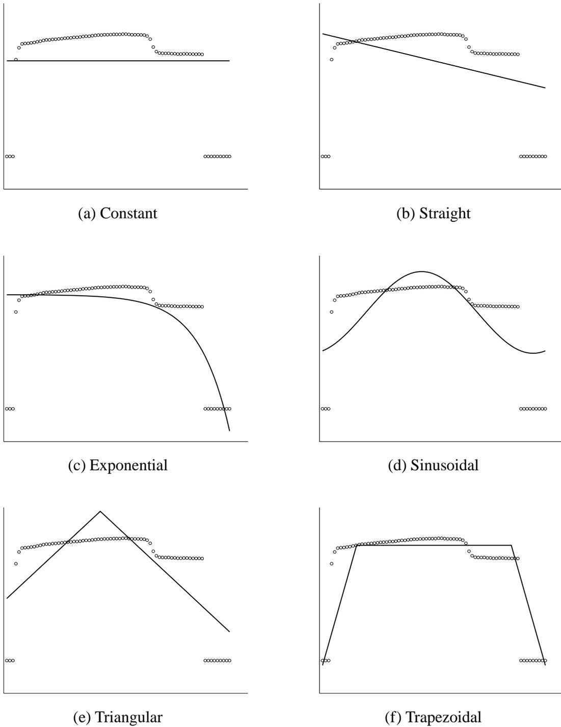
**Figure 3.1** The six structures fitted to a common data set. Each graph shows the input time-series data plotted with hollow bullets overlaid with a solid line representing one of the six structures. Each structure is fitted to the data so as to minimize the sum of squared error. The structures ordered from best to worst fit (i.e., from smallest to largest sum of squared error) are (f) trapezoidal, (e) triangular, (c) exponential, (d) sinusoidal, (b) straight, and (a) constant.
