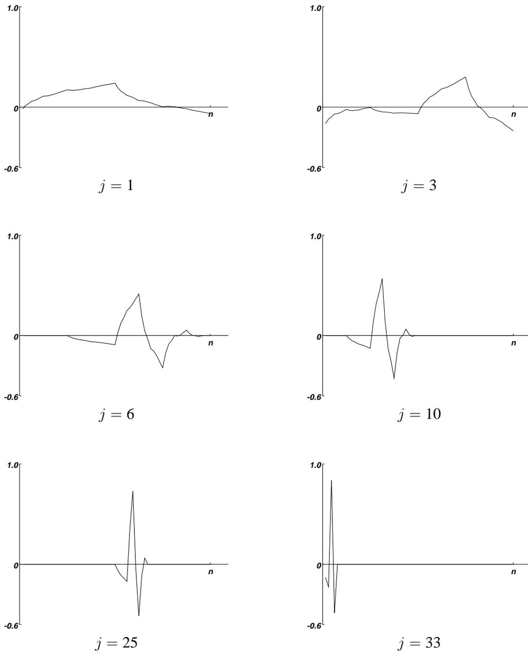
**Figure 4.3** A subset of the basis waveforms used by the wavelet transformation derived from the Daubechies 4-coefficient mother wavelet. The basis waveforms are ordered according to their degree of localization and indexed by  $j$  where  $j = \{0, 1, 2, \dots, n\}$  and  $n$  is the length of the data set. The basis waveforms with  $j$  equal to 1, 3, 6, 10, 25, and 33 are shown. Notice that as  $j$  increases, the basis waveforms become more localized.
