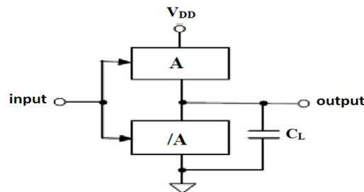
**Fig.1** Conventional CMOS logic circuit with pull-up (A) and pull down (/A) network
