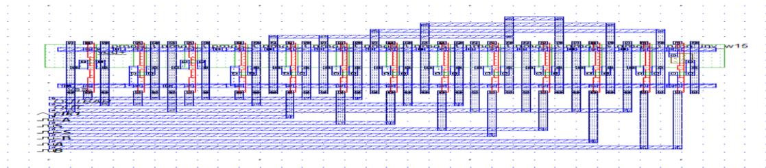
Fig. 11 Layout of proposed 2:1 Multiplexer.
