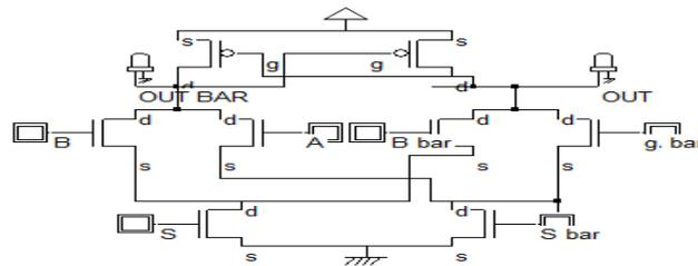
Fig. 4 Schematic design of DCVSL 2:1 Multiplexer [9].
