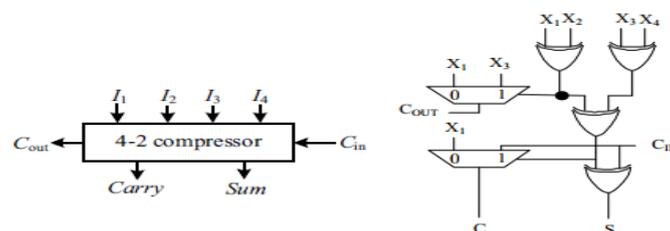
**Fig. 3** 4-2 Compressor using XOR and Multiplexer [6]
