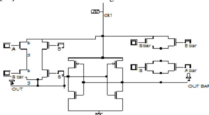
Fig. 8 Schematic design of proposed 2:1 adiabatic multiplexer.
