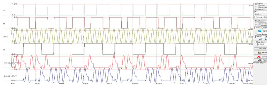
Fig. 12 Layout simulation of proposed 2:1 Multiplexer.
