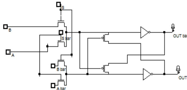
Fig. 7 Schematic design of EEPL 2:1 Multiplexer [10].
