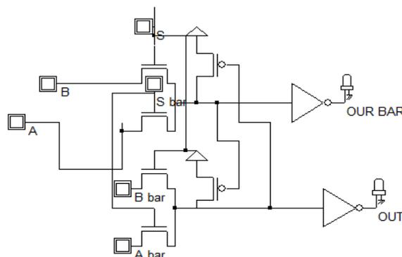
Fig. 6 Schematic design of CPL 2:1 Multiplexer [10].
