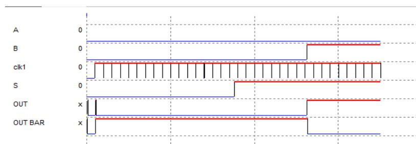
Fig. 9 Timing diagram of proposed 2:1 adiabatic multiplexer.
