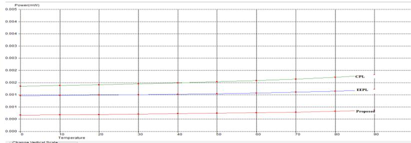
Fig. 18 Variation of power consumption with temperature for different Multiplexer at 1.2V
