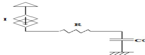
**Fig. 2** Equivalent model during charging process in adiabatic circuits.
