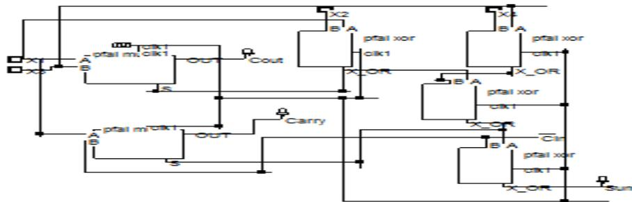
Fig. 10 Adiabatic multiplexer based 4-2 compressor.
