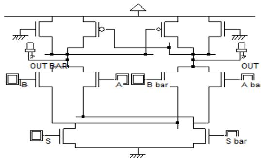
Fig. 5 Schematic design of MDCVSL 2:1 Multiplexer [9].
