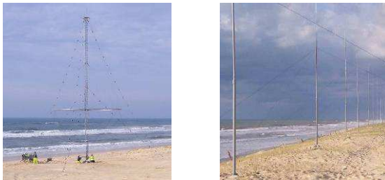
Figure 4 - Prototype du radar HFSW de l'ONERA
