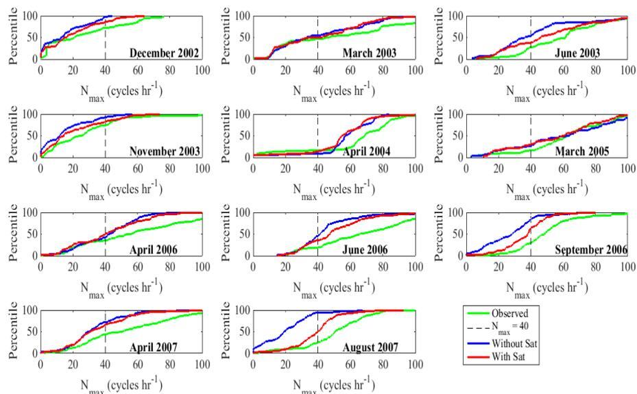
**Figure 9.** Cumulative distribution function of maximum buoyancy frequency ( $N_{\max}$ ), which is an index of the strength of vertical stratifications, for 12 cruises (20–90 stations occupied per cruise from December 2002 to August 2007). Observations (green) were compared to a reference model run without satellite data (blue) and a test model run with satellite data (red). The black dashed vertical line at  $N = 40$  represents the buoyancy frequency at which hypoxia begins to occur [7].
