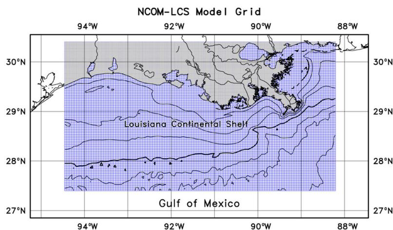
**Figure 1.** NCOM-LCS model domain and grid (every second gridline shown). The model ocean topography is contoured.
