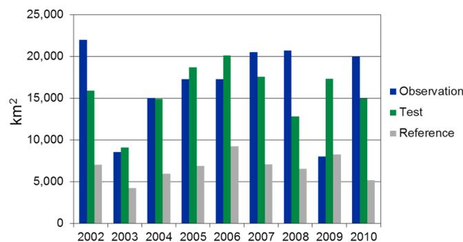
**Figure 11.** Area of bottom hypoxia on the Louisiana Shelf: blue from observation, green from the test case with satellite data and grey from the reference case without satellite data. For the model, the hypoxic area was estimated as the area where the hypoxic condition ( $\text{DO} < 64 \text{ mmol/m}^3$ ) persisted over 15 days each season.
