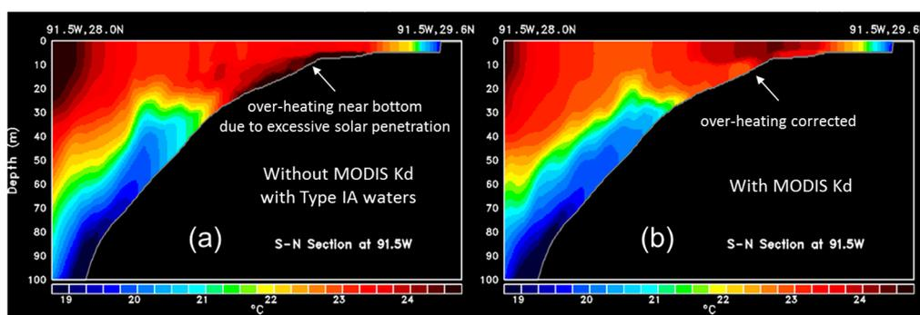
**Figure 7.** Effect of including satellite diffuse attenuation coefficient ( $K_d$ ) on thermal structure. Temperature north-south cross-section (right to left) at  $91.5^\circ\text{W}$  for May 2008 for (a) reference run (solar attenuation parameterized as Jerlov Type 1A oligotrophic water); and for (b) test run (solar attenuation determined from satellite  $K_d$ ).
