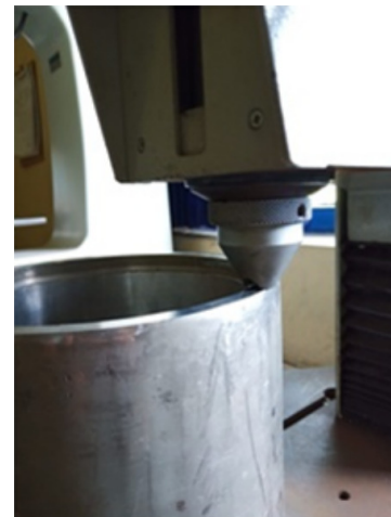
FIGURE 3. Rockwell hardness test with ball indenter.
