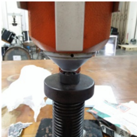
FIGURE 2. Brinell hardness test.
