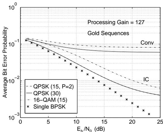
Fig. 7. Comparison between a parallel channel QPSK system and asynchronous 16-QAM and QPSK systems.
