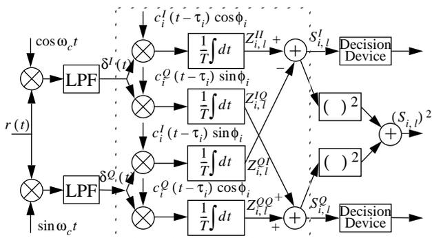
Fig. 1. M-ary QAM DS/CDMA receiver.
