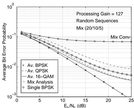
Fig. 5. Performance of mixed modulation system with and without IC under Rayleigh fading.
