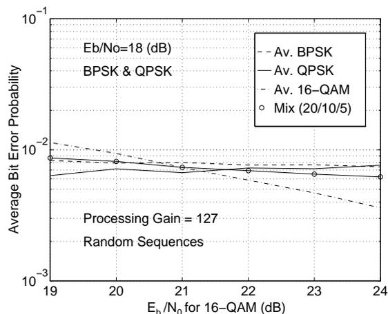
Fig. 6. Performance of mixed modulation system under fading with users employing different power levels.
