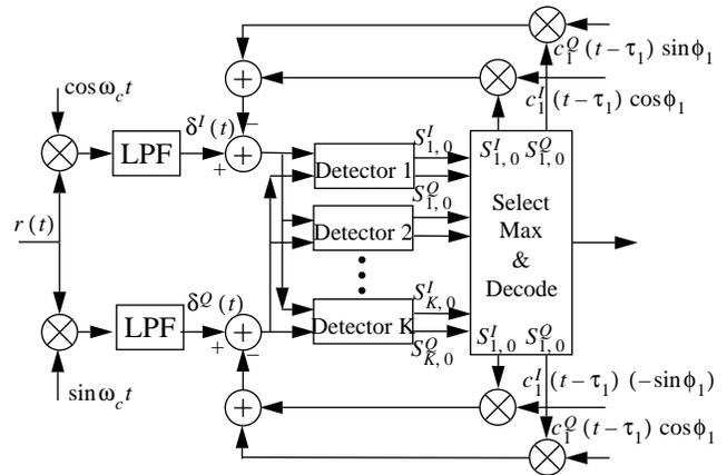
Fig. 2. M-ary QAM receiver with IC.
