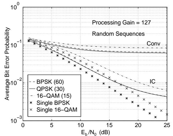
Fig. 4. Performance of single modulation systems with and without IC under Rayleigh fading.
