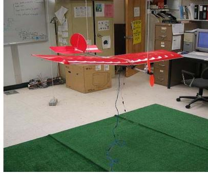
Fig. 3: Low-altitude test setup with the aircraft suspended at the nose and tail for adjustable pitch and altitude
