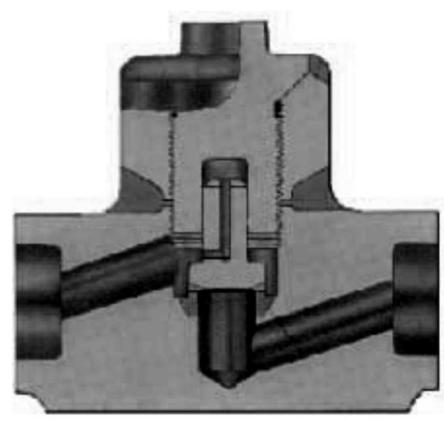
Fig. 3 : Cross section of Body Yoke Weld joint
