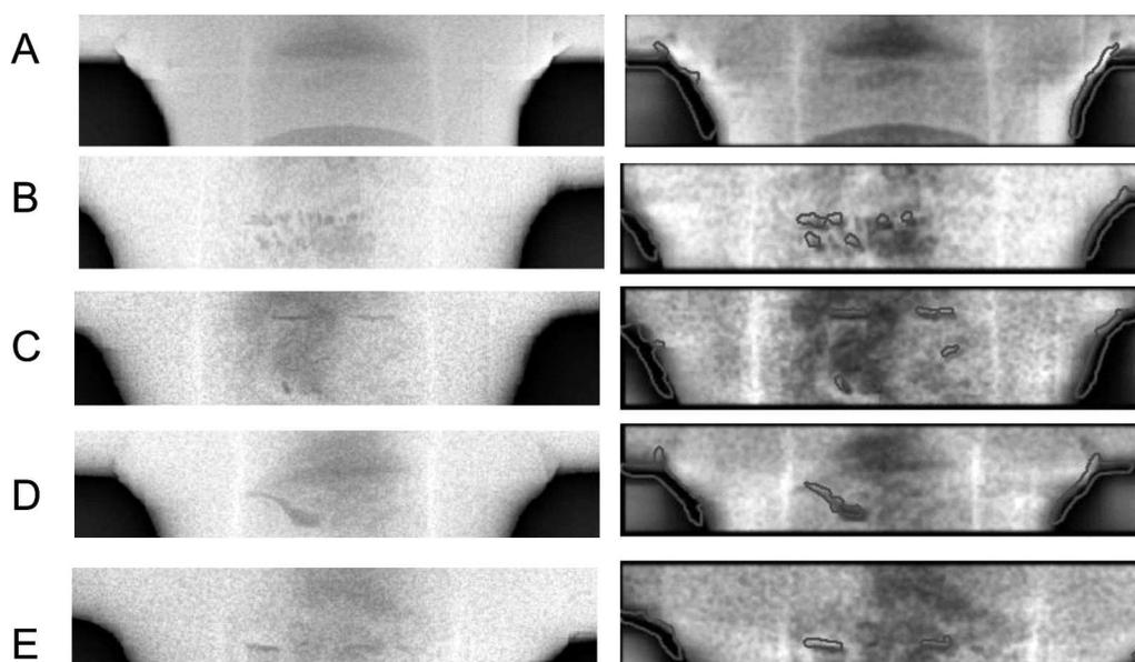
Fig. 12 : The results from the ADR software with the images on left side and ADR results superimposed on the images on the right side for different valve images (A) No Defect, (B) Cluster of porosity, (C) Planar Defect and gas holes, (D) Slag, (E) Planar Defect.
