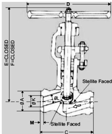
Fig. 1 : Structure of Hancock Valve welds
