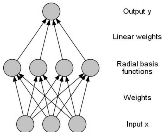
Fig. 10 : Structure of RBF Neural Network
