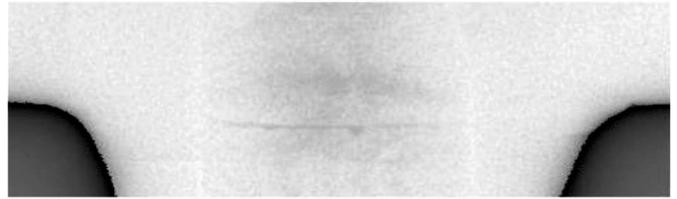
Fig. 7 : RoI (Weld Region) after Segmentation
