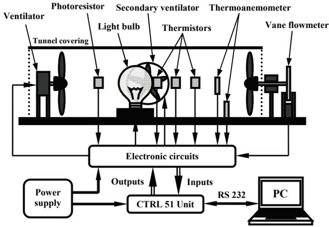
Fig. 5. Scheme of hot-air tunnel and whole control system
