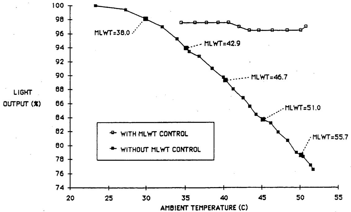
Figure 4. Light output vs ambient temperature, with and without controlling MLWT.
