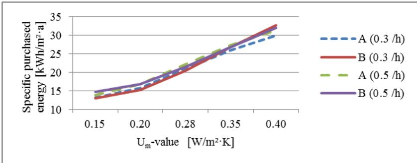
Fig.6 Specific purchased energy for system A and B varying with U<sub>m</sub>-value and air change rate (L)
