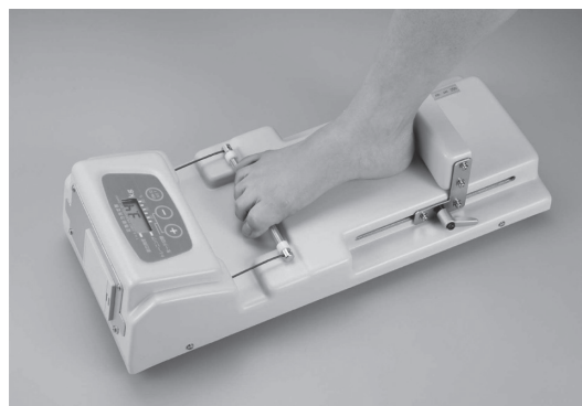
Fig. 1. Test of toe grip strength. The first proximal phalanx is positioned on the grip bar and the movable heel stopper is adjusted to fit the heel.
