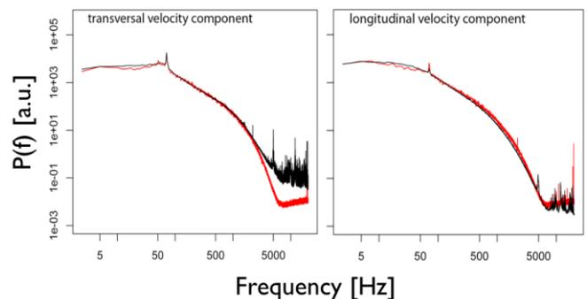
**Fig. 2** Comparison of power spectra for the longitudinal and transversal velocity component of the 2D-LCA (black) and an x-wire (red).
