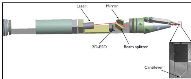
**Fig. 1** Setup of the 2D-Laser Cantilever Anemometer
