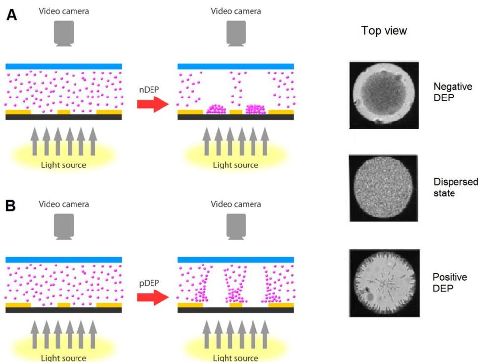
A circular “ring-dot” electrode geometry was proposed by Taff and Voldman for bioparticle trapping and sorting using p-DEP [73]. The ring-dot electrode geometry incorporates an outer ring
