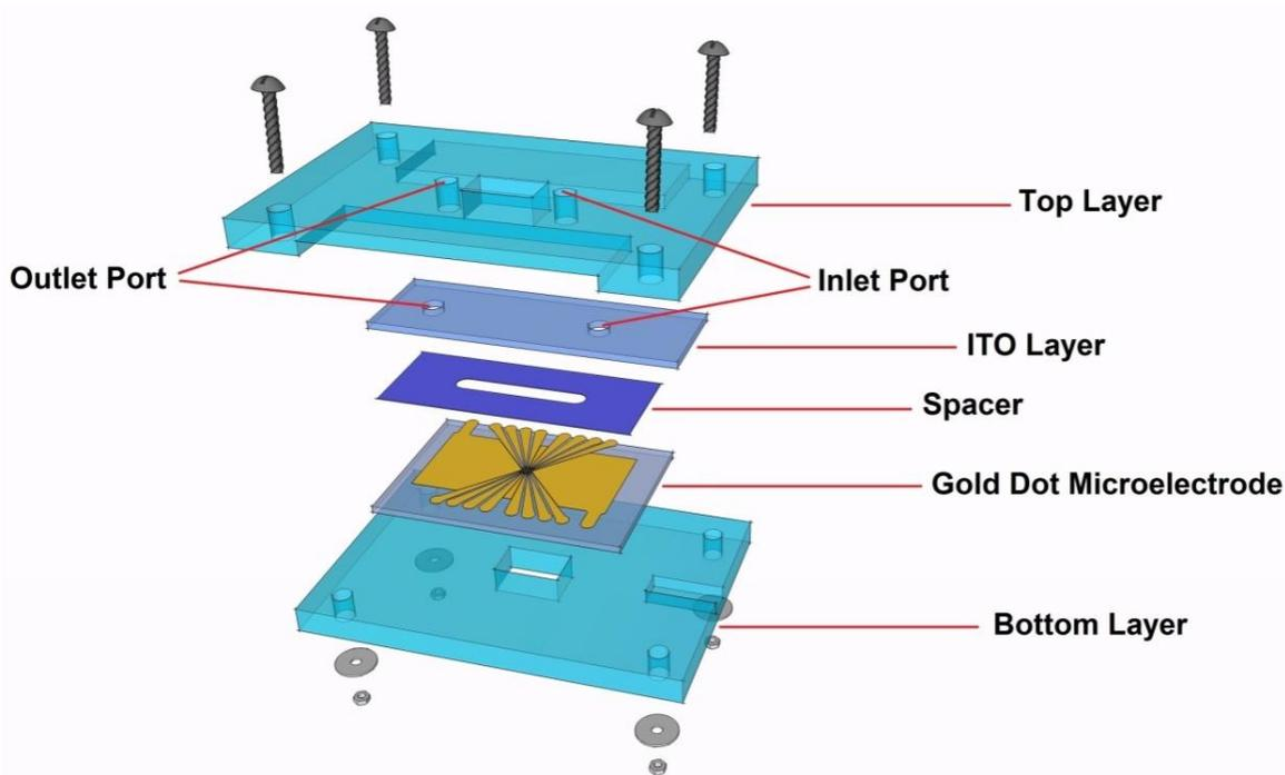
**Table 2.** Design specifications of the different layers of the proposed LOC device.
