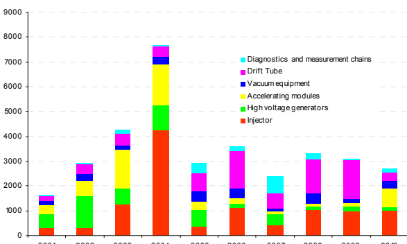
Figure 3: Corrective operation time per year for the whole AIRIX machine. 2001 is incomplete; the database was started after mid-year.
