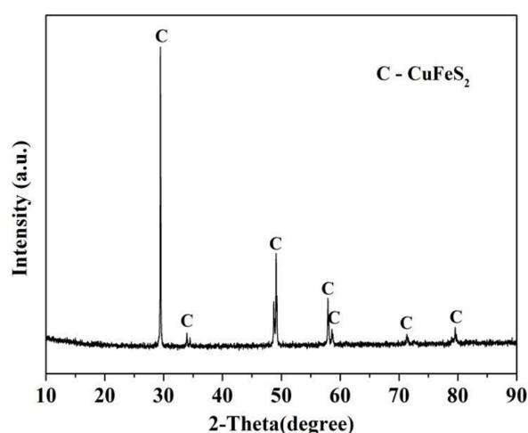
Figure 1. X-ray Diffraction patterns of chalcopyrite.
