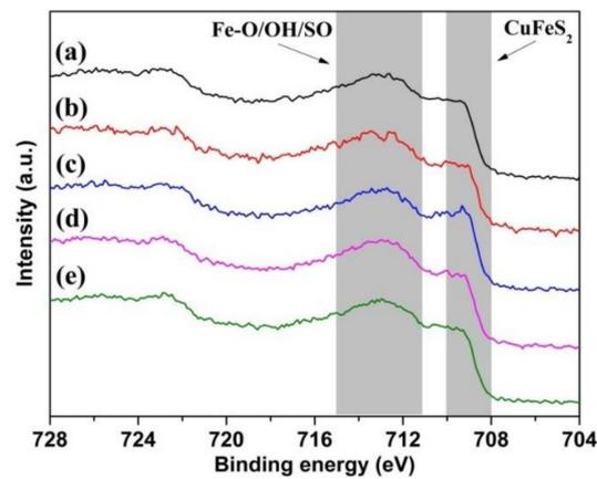
**Figure 13.** Fe 2p XPS spectra of (a) untreated chalcopyrite and chalcopyrite treated in (b) 0.01 M CaCl<sub>2</sub>, (c) 0.01 M CaCl<sub>2</sub> + 10 mg/L SHMP, (d) 0.05 M MgCl<sub>2</sub> and (e) 0.05 M MgCl<sub>2</sub> + 10 mg/L SHMP.
