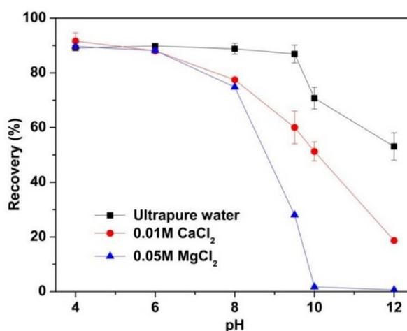
Figure 2. Chalcopyrite recovery as a function of pH.
