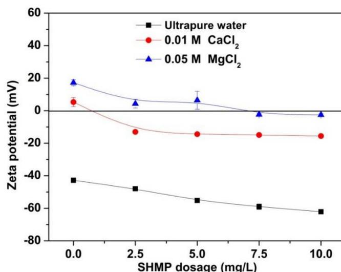
Figure 6. Zeta potential of chalcopyrite in the presence of SHMP at pH 9.5.
