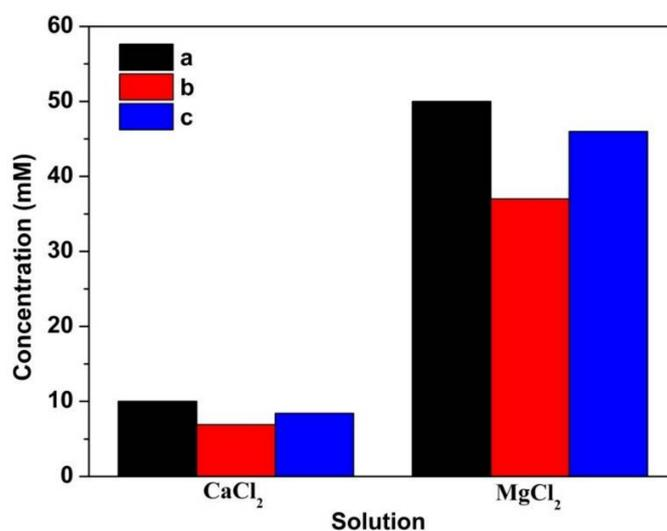
**Figure 7.** Concentrations of dissolvable Ca and Mg species in the flotation cell, (a) before flotation, (b) after flotation, (c) after flotation with SHMP.
