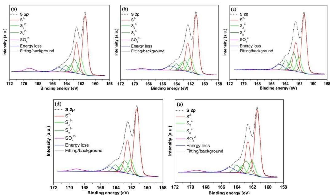
**Figure 10.** S 2p XPS spectra of (a) untreated chalcopyrite and treated in (b) 0.01 M CaCl<sub>2</sub>, (c) 0.01 M CaCl<sub>2</sub> + SHMP, (d) 0.05 M MgCl<sub>2</sub> and (e) 0.05 M MgCl<sub>2</sub> + SHMP.
