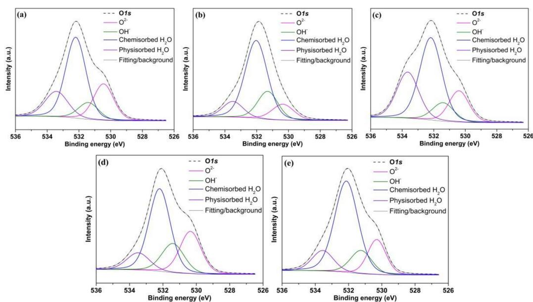
**Figure 11.** O 1s XPS spectra of (a) untreated chalcopyrite and chalcopyrite treated in (b) 0.01 M CaCl<sub>2</sub>, (c) 0.01 M CaCl<sub>2</sub> + 10 mg/L SHMP, (d) 0.05 M MgCl<sub>2</sub> and (e) 0.05 M MgCl<sub>2</sub> + 10 mg/L SHMP.
