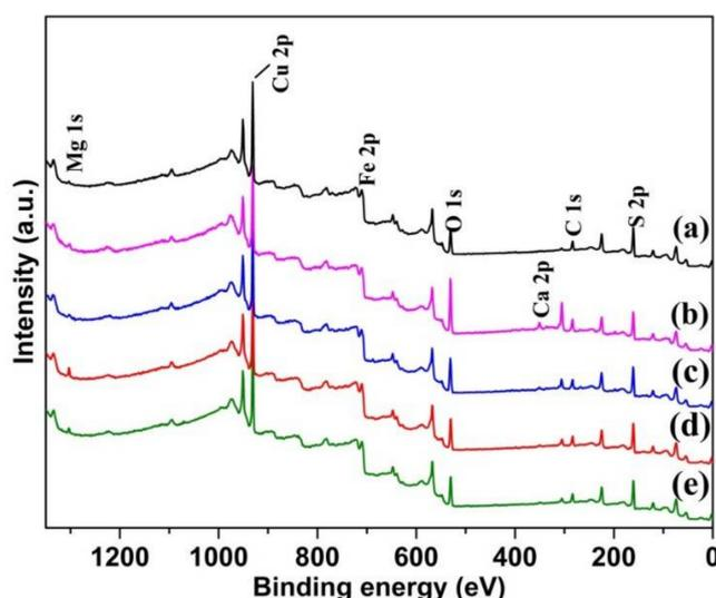
**Figure 9.** XPS survey spectra of chalcopyrite, (a) untreated, treated in (b) 0.01M  $CaCl_2$ , (c) 0.01M  $CaCl_2$  + SHMP, (d) 0.05 M  $MgCl_2$ , (e) 0.05 M  $MgCl_2$  + SHMP.
