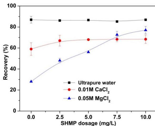
Figure 3. Effects of SHMP dosage on chalcopyrite recovery at pH 9.5.
