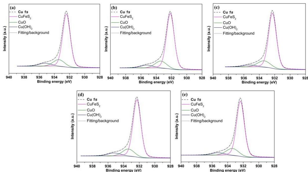
**Figure 12.** Cu 2p XPS spectrum of (a) untreated chalcopyrite and treated in (b) 0.01 M  $\text{CaCl}_2$ , (c) 0.01 M  $\text{CaCl}_2 + \text{SHMP}$ , (d) 0.05 M  $\text{MgCl}_2$  and (e) 0.05 M  $\text{MgCl}_2 + \text{SHMP}$ .
