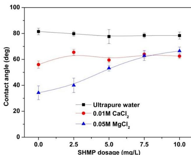
Figure 5. Contact angle of chalcopyrite in the presence of SHMP at pH 9.5.
