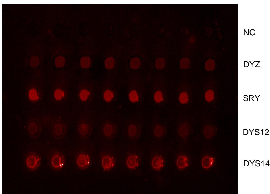
NC = signal obtained from negative control primer; the four rows of spots below the control in the picture denoted the amplification result of DYZ, SRY, DYS12 and DYS14 respectively.
