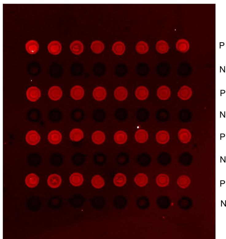
The spots in the picture show the amplification result of the positive and negative primers on the slide. P denoted the spots of each row were positive primer and N denoted the spots in the row were negative primer.
