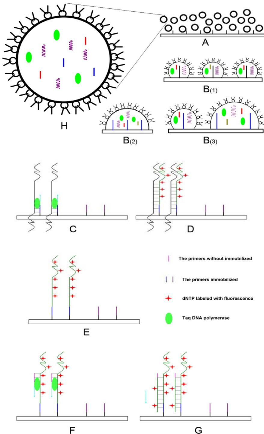
In the picture A denotes the first step of on-chip PCR, when emulsion was simply added to the surface of slide. B(1), B(2) and B(3) show three possible emulsion phase primer states and the other PCR component have been released to the slide. C to G described the role of primers and template on the slide in the first two cycles of on-chip PCR, Cy5 labeled dUTP was incorporated at each extension step. H denotes the typical water in oil emulsion system.
