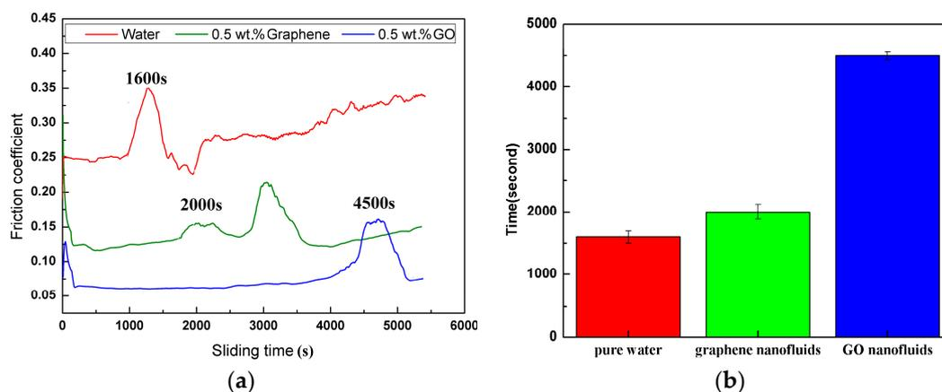
**Figure 7.** Sliding time to lubrication-film breakdown (a) and the average time of the lubrication films fails; (b) (8 N, 0.03 m/s, 90 min).
