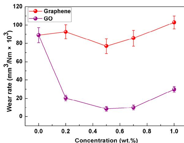
**Figure 4.** The average wear rate as a function of nanoparticles concentration in water (3 N, 0.08 m/s, 30 min).
