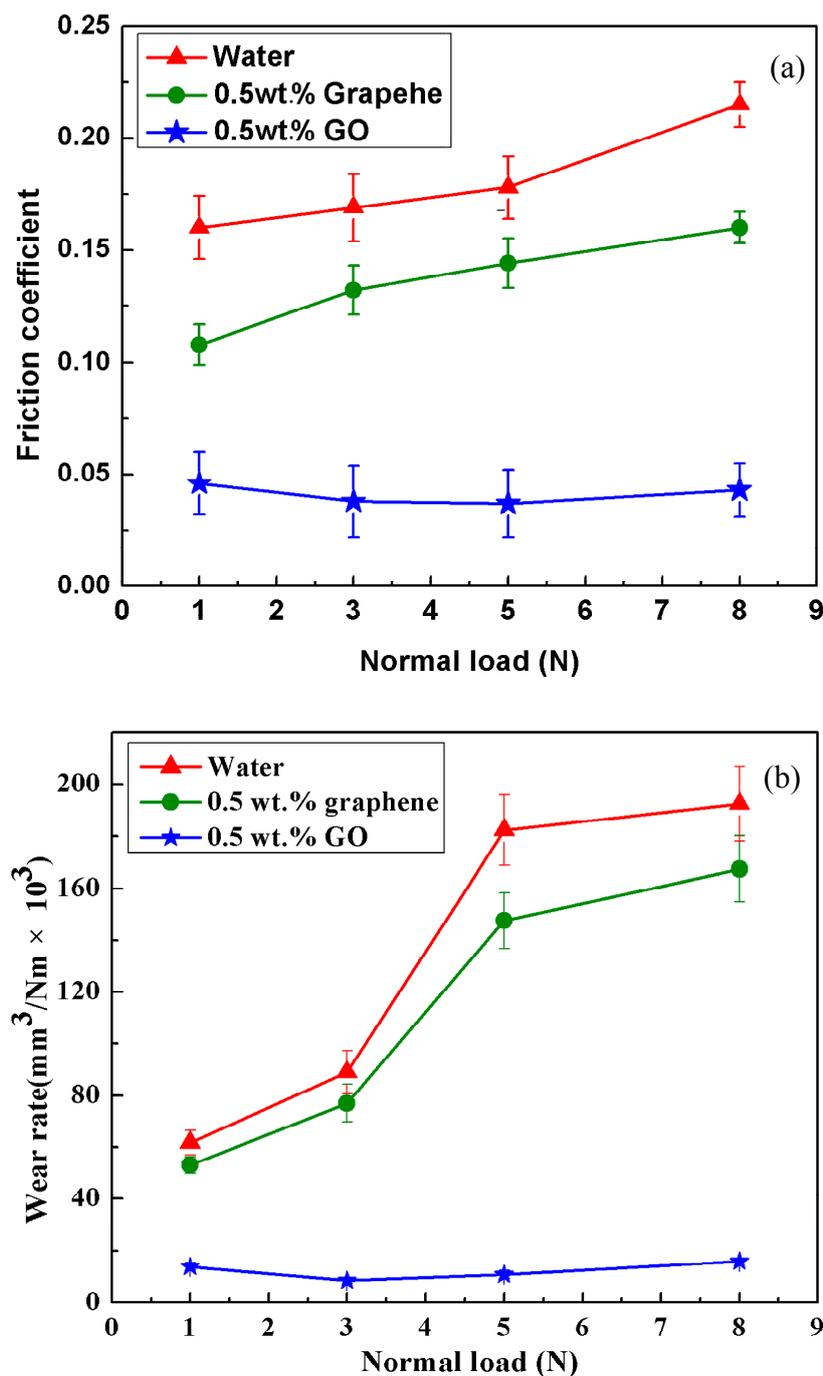
**Figure 6.** Effects of loads on average friction coefficient (a) and wear rate (b) of magnesium alloy specimens lubricated by the water with and without nanoparticles (0.08 m/s, 30 min).
