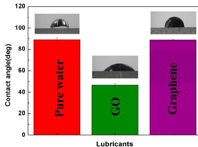
**Figure 8.** The contact angle of AZ31 magnesium alloy surface for pure water, 0.5 wt.% graphene nanofluids and 0.5 wt.% GO nanofluids.
