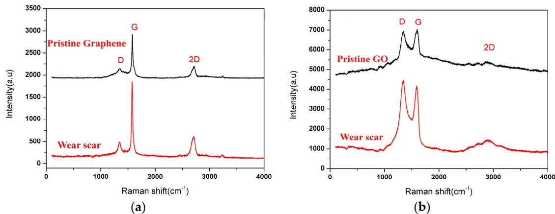
**Figure 10.** Raman results for the wear surface lubricated with (a) 0.5 wt.% graphene nanofluids; (b) 0.5 wt.% GO nanofluids (3 N, 0.08 m/s, 30 min).
