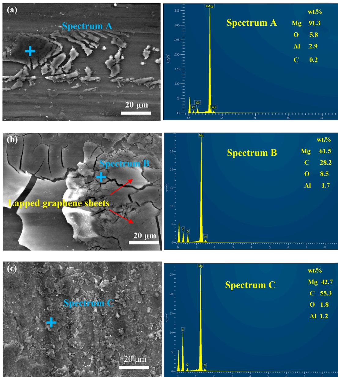
**Figure 9.** FESEM-EDS results for the wear surface lubricated with (a) pure water; (b) 0.5 wt.% graphene nanofluids; (c) 0.5 wt.% GO nanofluids (3 N, 0.08 m/s, 30 min).
