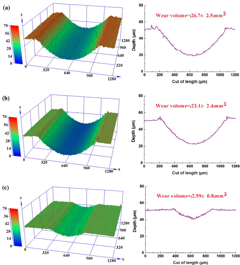
**Figure 5.** 3D topography images and 2D profiles across the wear tracks for flat specimens after wear tests with (a) pure water; (b) 0.5 wt.% graphene nanofluids; (c) 0.5 wt.% GO nanofluids (3 N, 0.08 m/s, 30 min).
