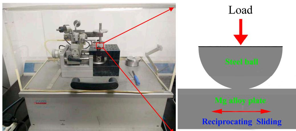
**Figure 2.** The ball-on-flat reciprocating sliding tester and schematic of ball-pot assembly in ball-on-flat tribotester.
