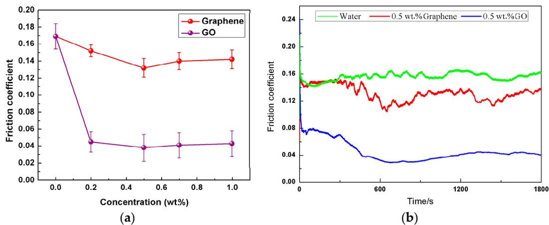
**Figure 3.** (a) The average friction coefficient as a function of nanoparticles concentration in water and (b) the friction coefficient relative to sliding time (3 N, 0.08 m/s, 30 min).
