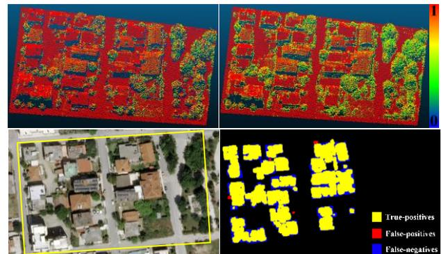
Figure 2. The LIDAR point cloud coloured by the initial  $N_z$  values (top left); the filtered  $N_z$  values by the scan line smooth filtering technique (top right); the orthoimage of the area of interest (bottom left) and the evaluation of the building detection results (bottom right).
