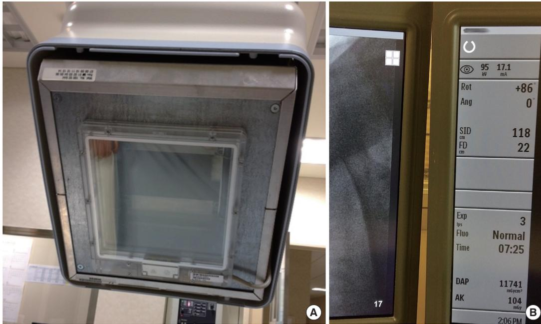
Fig. 3. Separate installed internal DAP meter (A) and display screen (B). There are DAP meters that can be installed in the fluoroscopy machine internally to monitor dose.
