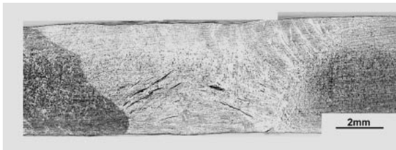
Fig. 14 An optical micrograph of fractured SNb1 specimen tested at 300°C.
