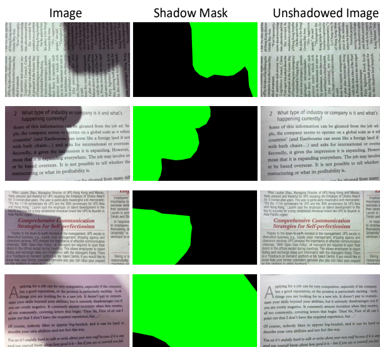
Figure 5. Some examples of the proposed dataset. Specifically, the middle column gives the shadow masks and the green areas indicate the shadow regions. The right column represents the ground truth.
