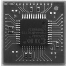
Fig. 2 Top view of the package with a CPLD
