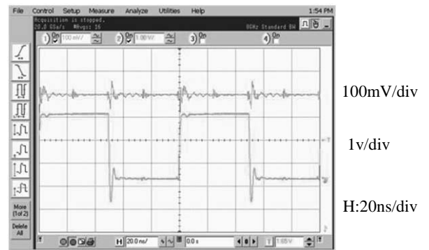
Fig. 8 Power-ground bounce (top) and output signal (bottom) and for the case with SMD capacitors.
