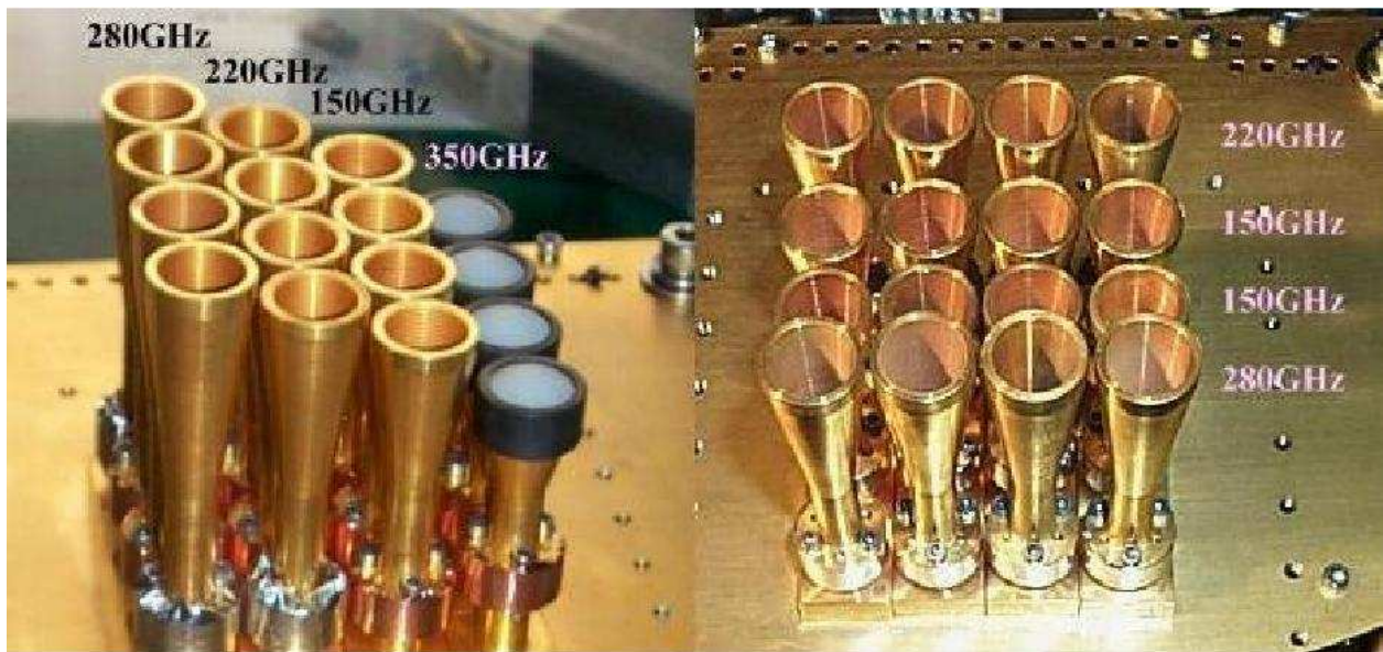
Fig. 1.— Images of the ACBAR focal plane layout for 2001 (left) and 2002 (right).
