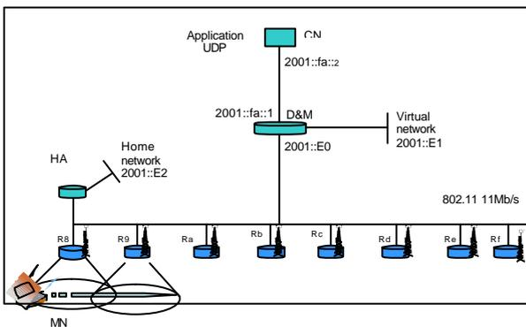
Figure 7: Simulation network topology.
