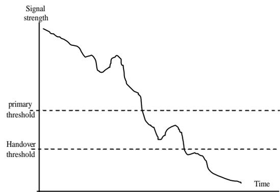
Figure 4: primary and handoff thresholds.
