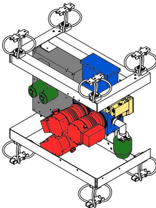
**Figure 2.** 3-D sketch of the compact PTR-ToF-MS as mounted in the P-3B flight rack. The color-coded components are as follows: thermostatted enclosure housing the glow discharge–ion drift tube (grey); ion transfer optics and ToF-MS flight tube (blue); turbomolecular pumps (red); pressure gauges (green) and electronic mass flow and pressure controllers (yellow).
