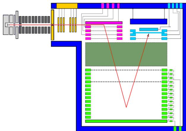
**Figure 1.** Schematic drawing of the newly developed compact PTR-ToF-MS instrument. The color-coded components are as follows: glow discharge (light grey), ion drift tube (dark grey), ion transfer optics (dark yellow), orthogonal ion accelerator (magenta), field-free time-of-flight region (olive green), double-stage ion mirror (light green), post-accelerator and multichannel plate (MCP) detector (light blue). The ion path is shown in red. Housing and mounting parts are shown in deep blue.
