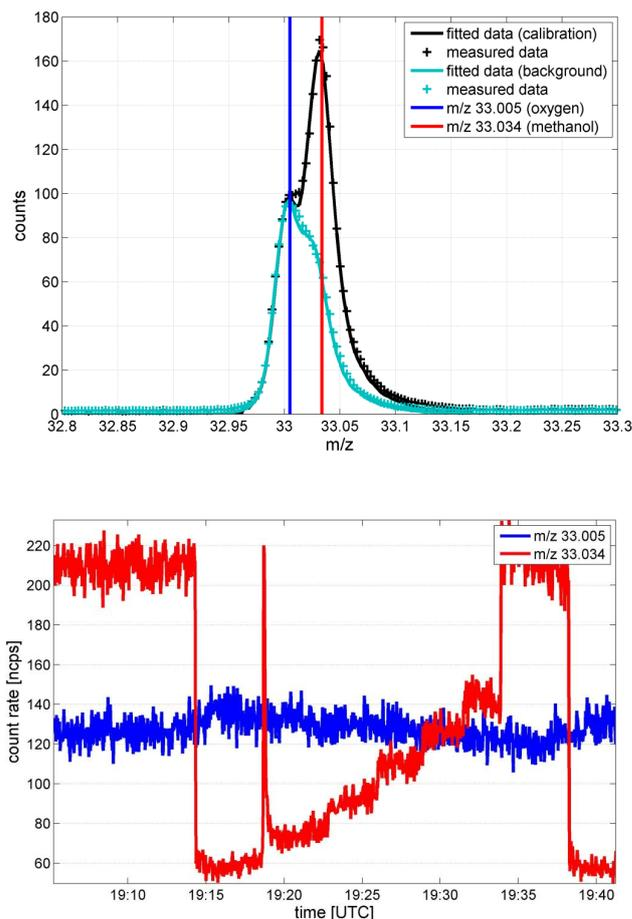
**Figure 4.** Resolution of isobaric  $HO_2^+$  ( $m/z$  33.005, protonated molecular oxygen) and  $CH_5O^+$  ( $m/z$  33.034, protonated methanol) ions in a 1 min average mass spectrum (top) and the time series of the two signals obtained during a multipoint calibration with methanol (bottom).
