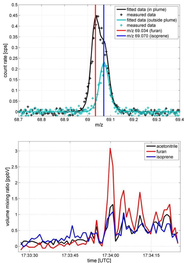
**Figure 5.** Resolution of isobaric  $C_4H_5O^+$  ( $m/z$  69.034, protonated furan) and  $C_5H_9^+$  ( $m/z$  69.070, protonated isoprene) ions (1 min signal average) measured in an agricultural crop-burning plume. The signal obtained outside the plume is included for comparison (top). Time series of furan, isoprene (for interferences see text) and acetoneitrile obtained during transect of an agricultural crop-burning plume on 23 September 2013 near Dublin, GA, USA (bottom).
