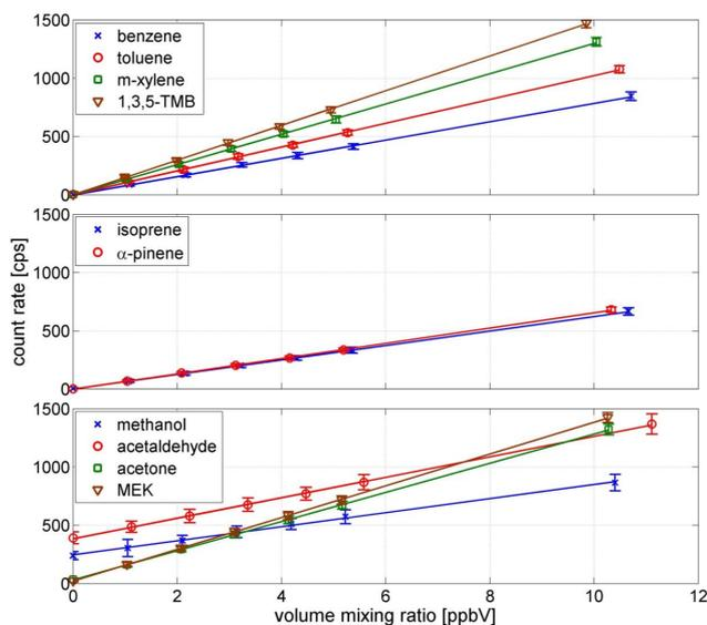
**Figure 3.** Calibration curves for aromatic VOCs (top), biogenic VOCs (center), and oxygenated VOCs (bottom). Signals measured are ion count rates at  $m/z$ s of the protonated molecules. Error bars indicate the precision of the 1 Hz data.
