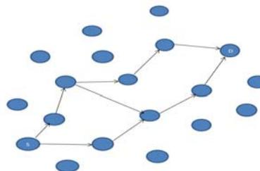
Fig.2. Restricted directional flooding in LAR and DREAM
