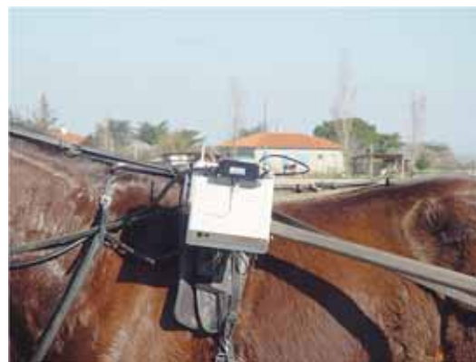
Fig. 3. A solid PVC box is fixed on the sulky.
