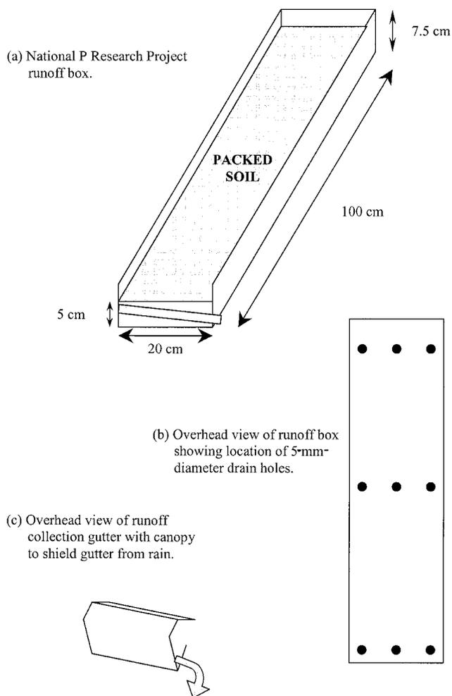
**Fig. 1.** Schematic diagram of runoff box used in this study including (a) overall dimensions, (b) drain holes in base of box, and (c) runoff collection gutter.
